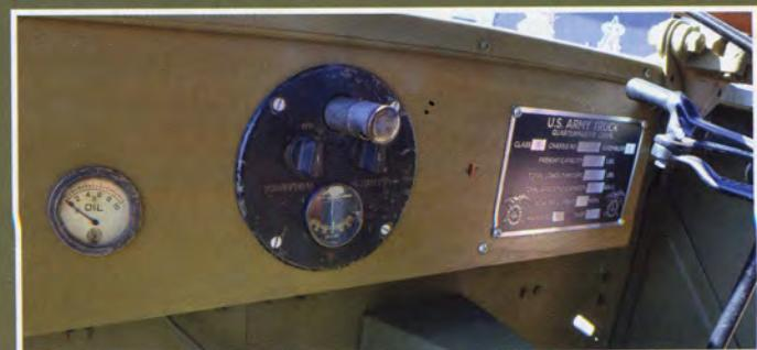
The spartan interior shows the height of technology from a century ago. The simple instruments comprises an oil pressure and amperage gage, along with switches for the ignition and lights.
