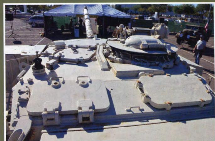
The Chieftain was armed with a 120mm rifled tank gun and a Coaxial L8A1 7.62 mm machine gun, and had an NBC protection system which Centurion lacked.
