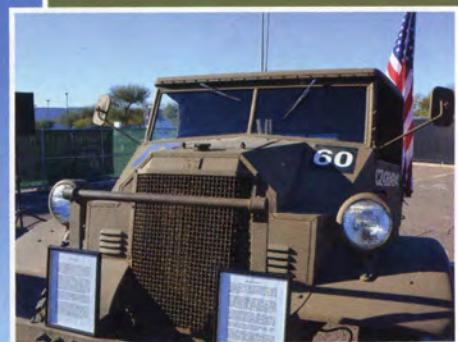
The first #11 cab designed at Ford by Sid Swallow is shown here. Ford-built truck grilles used a square mesh while Chevrolet-built vehicles had a diamond pattern.
