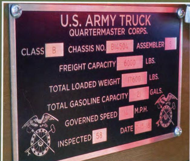
The data plate indicates a total loaded weight of 17600lbs allowing for 6000lbs of cargo. The fuel capacity is 21 gallons and the delivery date is listed as 7-15-18.
